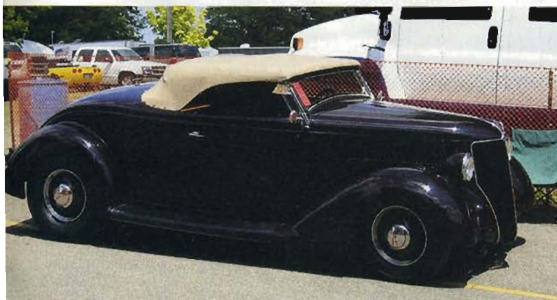
Rick Moe's '36 Ford roadster just oozes tradition, from its 4-inch chop and maroon paint, to the vintage 283 Chevy V-8, '39 Merc trans, and '40 Ford rear with a Hallbrand quick-change center. The rubber rake comes courtesy of 6.00-16 and 7.50-16 bias-plies.
