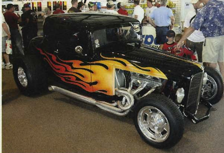
Vescio's Customizing and Restoration was showing off one of its latest creations—Steve Andersen's hot Deuce five-window. The chopped, sectioned, channeled, and stretched coupe rides on a Deuce Steel frame with SO-CAL suspension parts, and sports a 575hp small-block Chevy with wild Mike Cooper headers. Chip Foosse did the flames.
