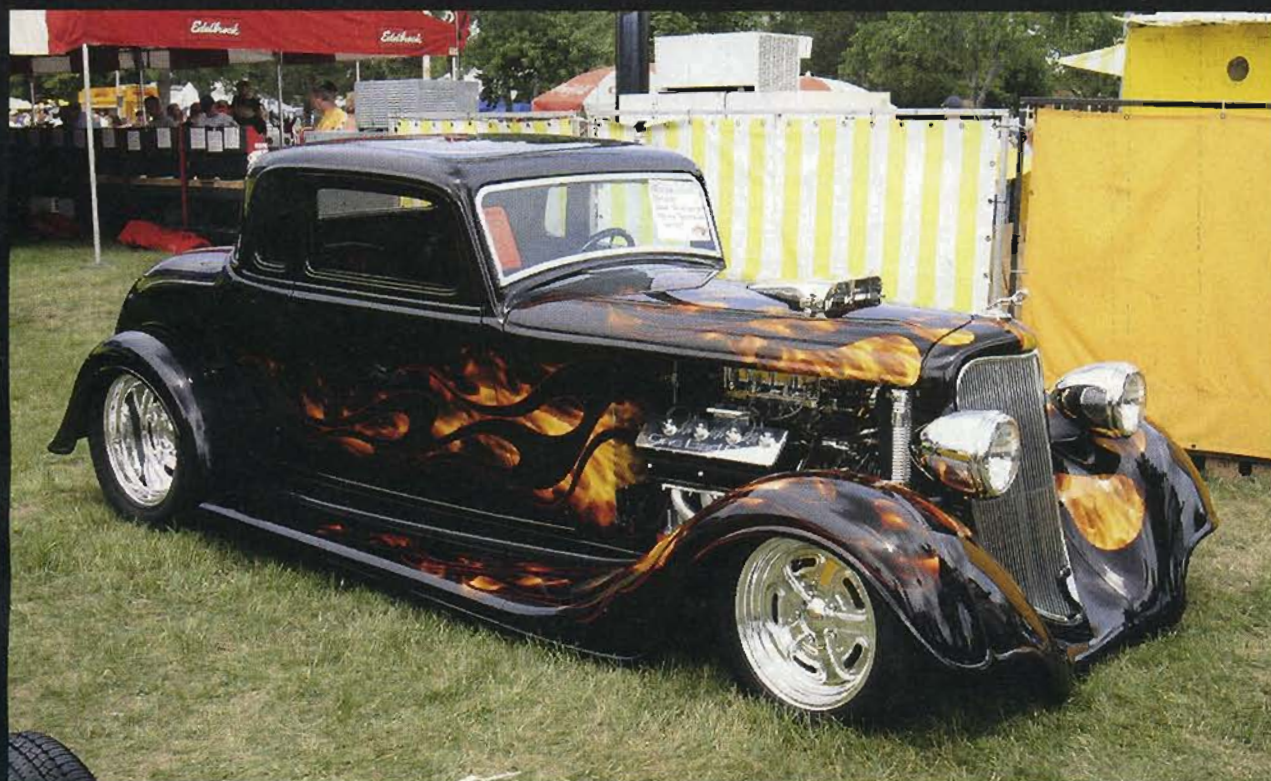
Norm Fey's '34 Dodge coupe is one badass Mopar, with a blown and injected 392 sending power through a Torqueflite to a narrowed Dana 60 rear. Realistic flames over black cherry paint and 16- and 18-inch Budnik rollers will keep you looking if you can pry your eyes from the mill.
